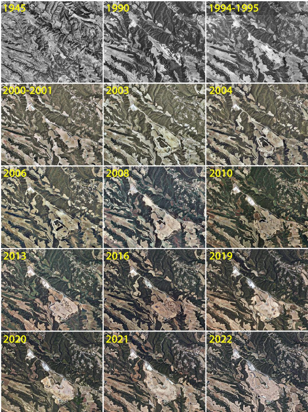
**Figure 18.** Orthophotos of the area of Can Mata showing the progressive development of the landfill over the years. Base orthophotomaps: © Institut Cartogràfic i Geològic de Catalunya, downloaded from VISSIR and reproduced with permission by means of a Creative Commons license CC BY 4.0.
